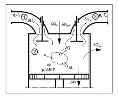
Fig. 1. Elementary processes in the engine cylinder and in the systems connected with it
